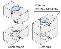
Decide the mounting hole position depending on the clamped part direction.
