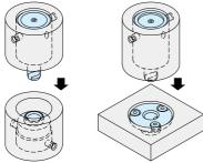
1. Align the cam groove with the ball in Locking Receptacle and insert.
